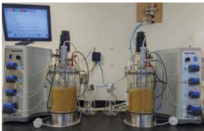
Two 10-litre fermentation tanks used to grow peptide expression bacteria.
